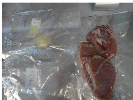
Figure 1. Meat package with the freshness sensors integrated
