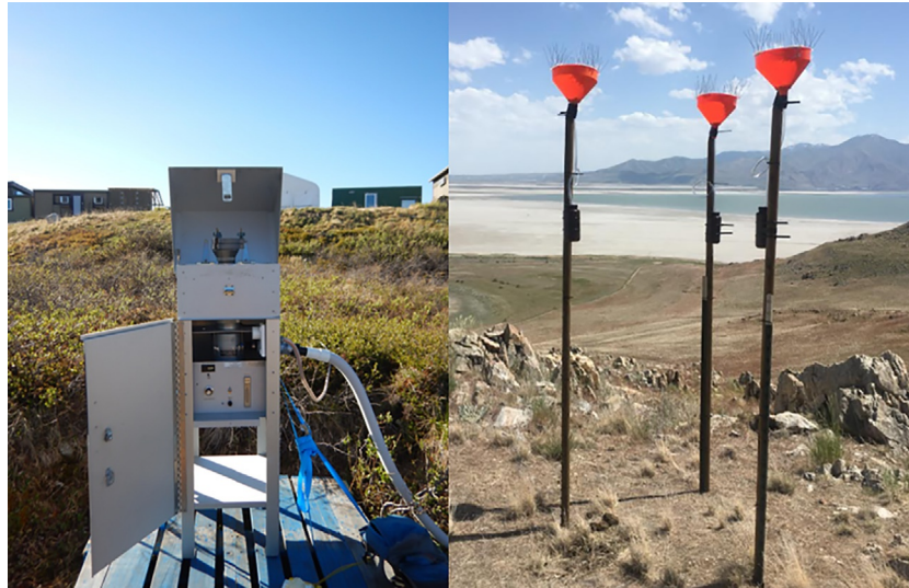
Fig. 6 Field deployed active (left) and passive deposition samplers. Photo credits: Jeff Perala-Dewey and Molly Blakowski.
