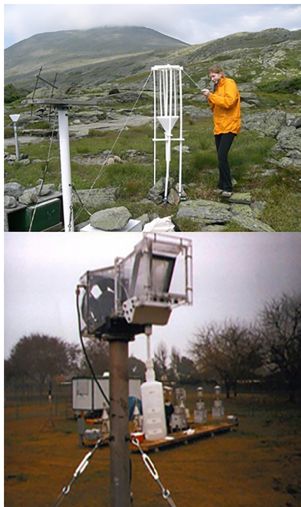
Fig. 7 Passive (top) and active sampling of fog. Photo credit: Kathleen Weathers (top), Collett research group (bottom).
