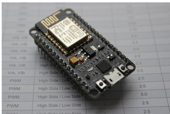
Figura 5.34: *NodeMCU v1.0*
