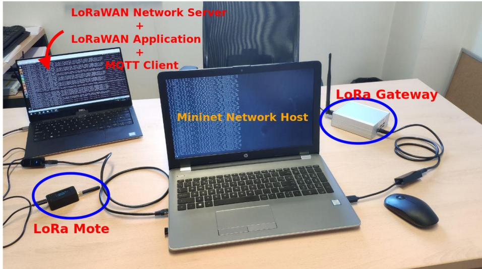
Figure 7.4: Setup of the physical test components.
